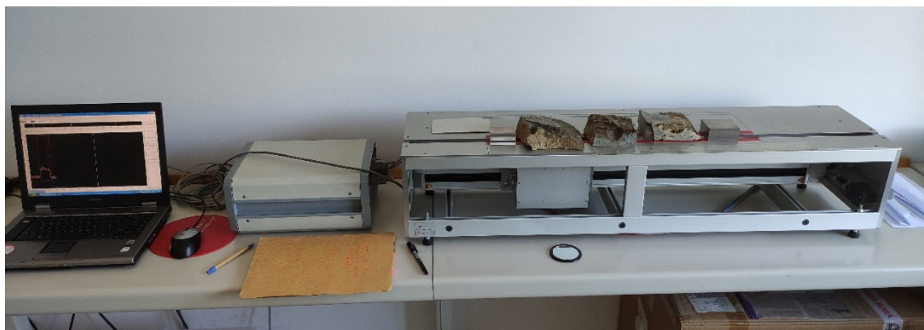
Fig. 4. The TCS device in a TC+TD mode with a set of rock samples along the scanning line (photo taken in 2022).
