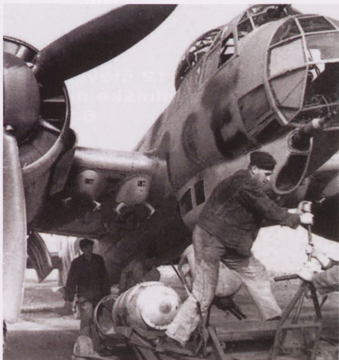
Ju 88 z dodatnim 20 mm topom MG FF v nosu
