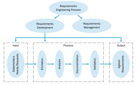
Figure 2 Requirements Engineering Process
