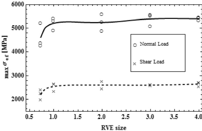
**Figure 2.** Max. effective stress for two loading cases depending upon RVE size
