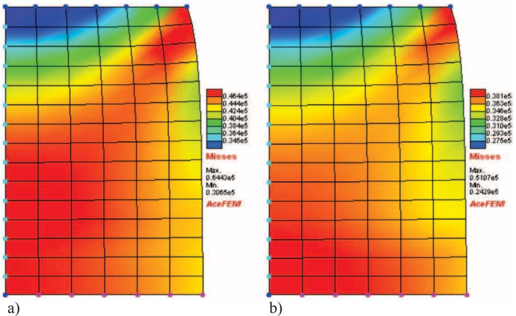
**Figure 5.** Effective stress in the macrostructure 2D a) stiff inclusions, b) voided microstructure.
