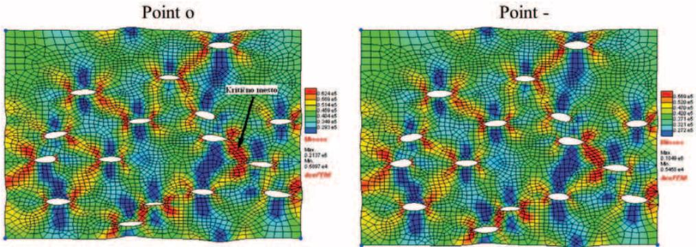
**Figure 6.** Effective stress in the RVE from the critical point of the macrostructure voided microstructure.
