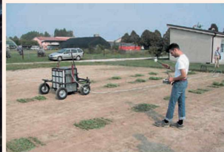
The microwave weed destroyer is an example of using knowledge derived from telecommunications in other fields to improve the quality of life. It makes it possible to kill weeds without the use of harmful chemicals. It was developed in cooperation with the University of Padua.
