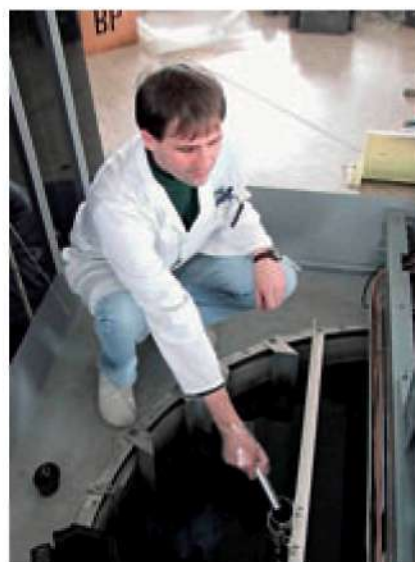
Dr Tomaž Žagar introducing a ceramic sample into the irradiation channel in the TRIGA Mark II.
