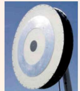
The "archery-target" antenna is a directional antenna evolved from the short-backfire antenna (SBFA). The new antenna has an additional annular reflector and a much-increased large reflector when compared to the SBFA. The new antenna is simple to manufacture, since the supporting structure for the small and annular reflectors can simultaneously serve as a radome.
