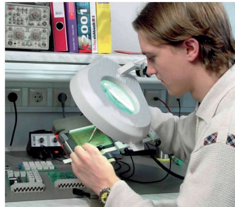
Elaboration of prototype printed circuit boards for the Cliniporator, the first European clinical device for the treatment of tumours by means of electrochemotherapy. The Cliniporator has been developed in collaboration with European partners at the Faculty of Electrical Engineering, University of Ljubljana, and in close collaboration with colleagues from the Institute of Oncology in Ljubljana.
