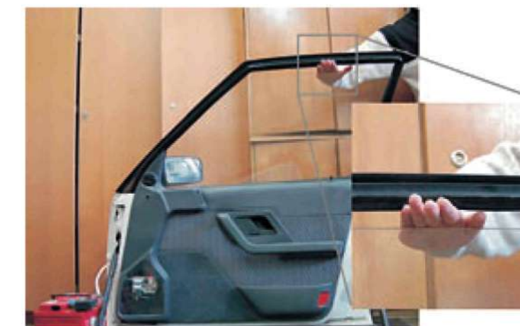
Fig. 8: Low-cost distributed fibre optic anti-squeeze sensors: effective protection against injuries caused by electric car windows.
