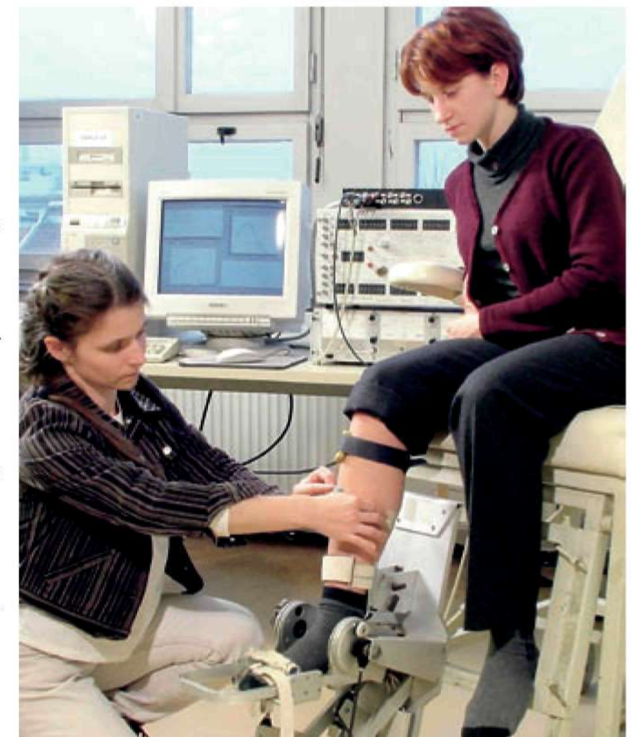
Dr Alenka Maček Lebar and Barbara Mali from the University of Ljubljana, Faculty of Electrical Engineering, during the measurement of electric activity of the muscle. Surface measurement of a muscle's electrical activity (electromyography) is a non-invasive technique used in diagnosis of muscle diseases and in training and testing of athletes.
