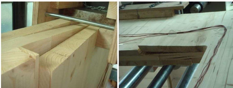
Slika 4.18: Porušni mehanizem nižje preklade – strig v zunanjih slojih in upogibna odpoved srednjega Figure 4.18: Failure mechanism of the lower beam – shear in outer layers and bending failure in the middle
