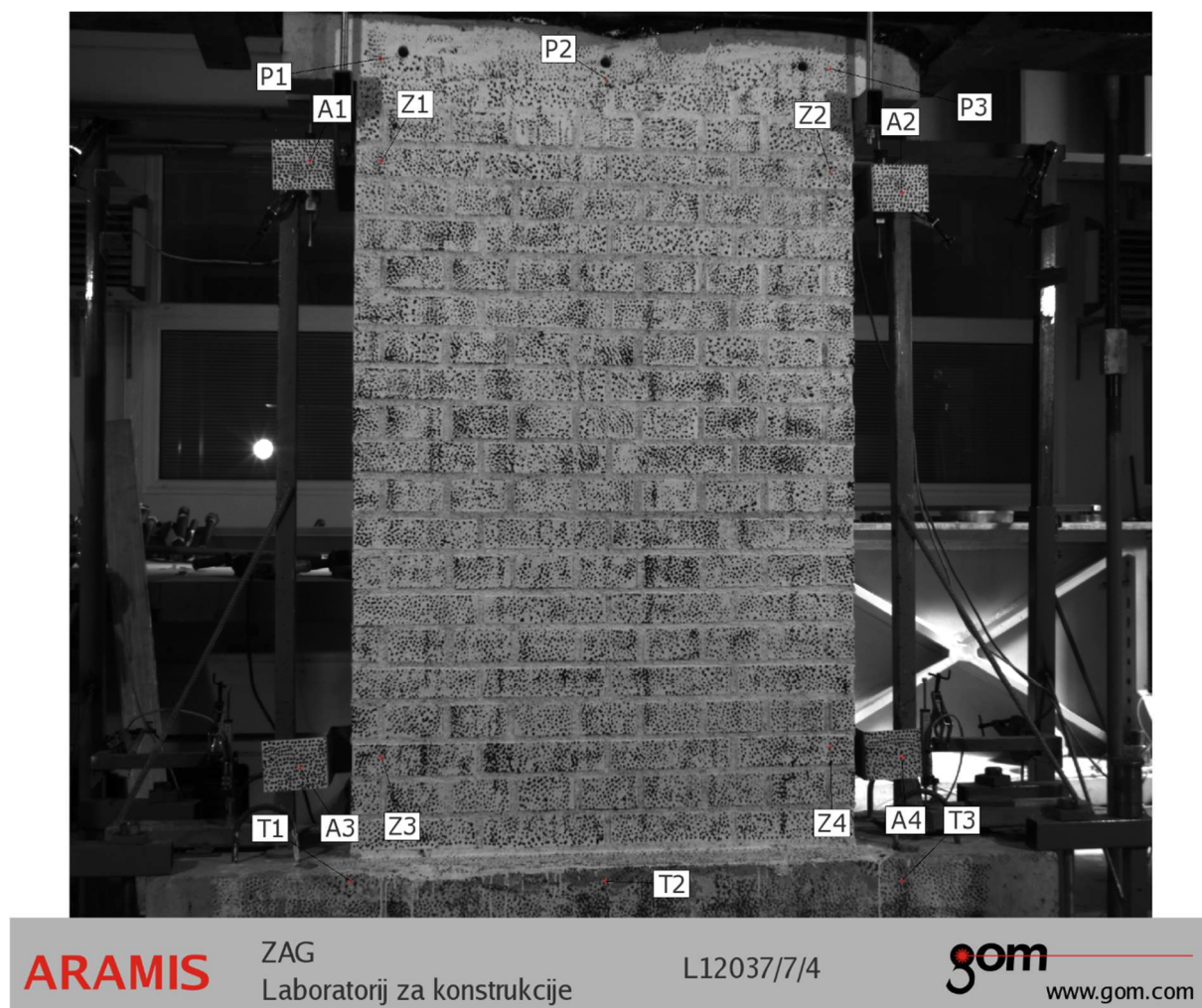
Slika B.6: Pozicije točk za fotografsko spremljanje pomikov opečnega zidu z ojačilno ploščo, privijačeno v zid Figure B.6: Positions of points for the photogrammetric displacement measuring of the wall with the strengthening plate mechanically bolted into the wall
