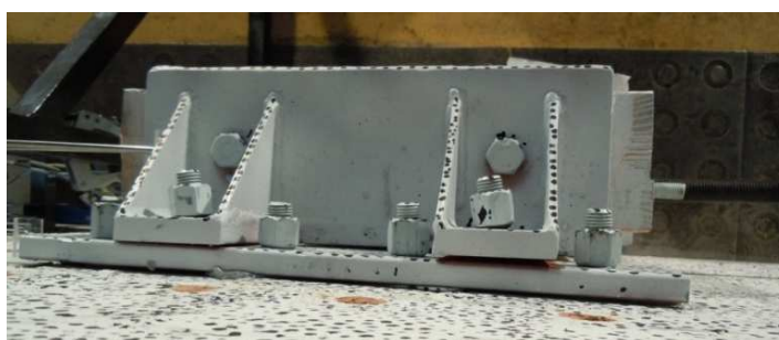
Slika 5.83: Porušni mehanizem – odpoved stika med čevljem in pločevino Figure 5.83: Failure mechanism – connection between the bracket and the metal plate
