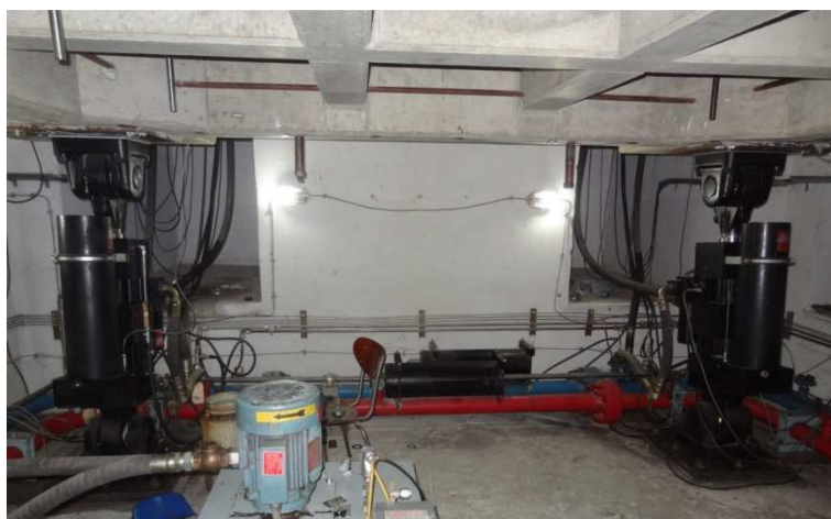
Slika 6.9: Dva od vertikalnih batov, na vrhu prednapeta AB platforma Figure 6.9: Two of the vertical actuators and the prestressed RC platform on top
