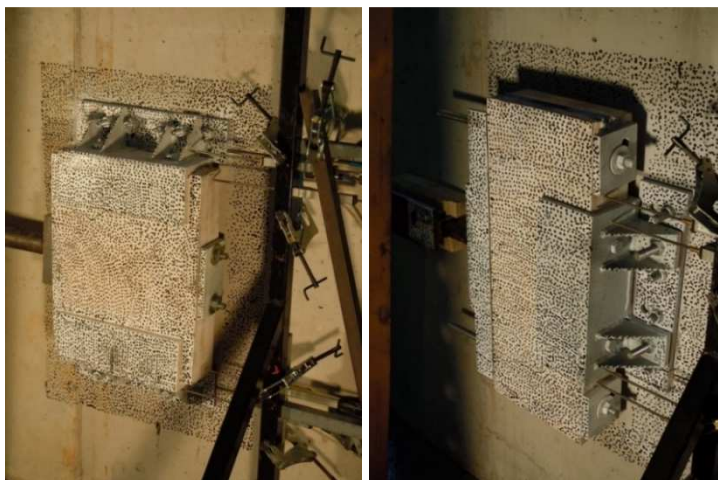
Slika 5.86: Horizontalni (levo) in vertikalni (desno) test spoja v betonu Figure 5.86: The horizontal (left) and vertical (right) test of the connection in concrete
