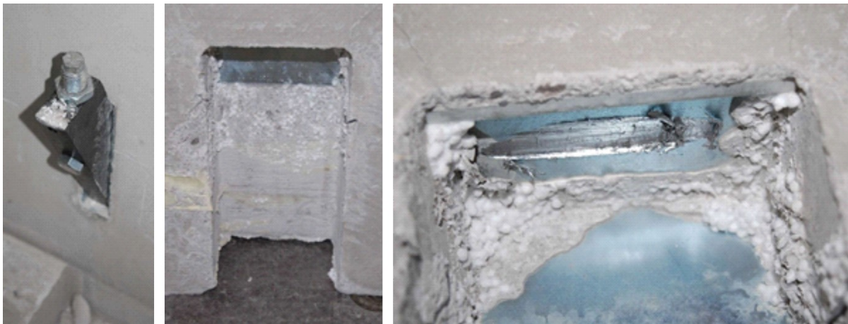
Figure 3.21: The significant material wear at the bottom connections observed during the experiments
