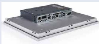
» Slika 10 - Automation Panel + IPC = Panel PC
