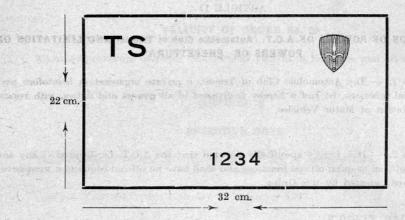
Description: Metal plates, 32 cm long, 22 cm high, with white background; Letters TS in upper left section; Numbers in lower section of plate from left to right, (8.5 cm high). Both letters and numerals to be black. A shield with red background to be on the upper right hand corner of plate, the center of which to bave an Alabard (Symbol of Trieste) imposed upon it in white; the shield to be 8 cm wide and 9 cm. 9 high.
