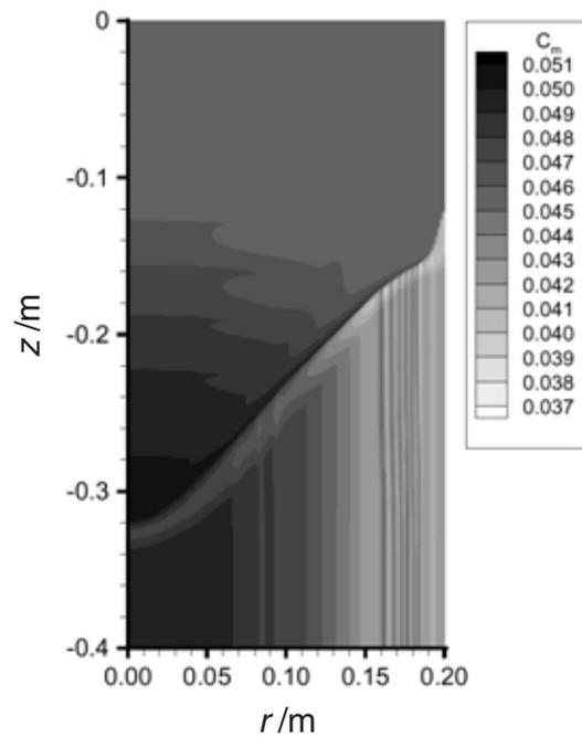
**Figure 4:** Mixture Cu concentration ( $C_m$ ) field in the billet
