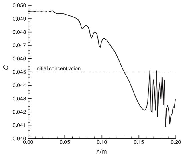
**Figure 5:** Radial Cu concentration profile in the solidified billet
