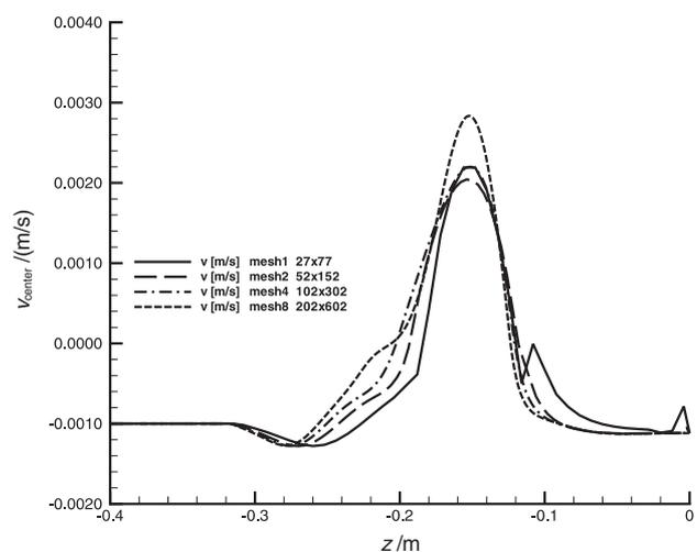
**Figure 1:** Vertical velocity component ( $v$ ) profiles along the billet centerline obtained in the computations without species transport
