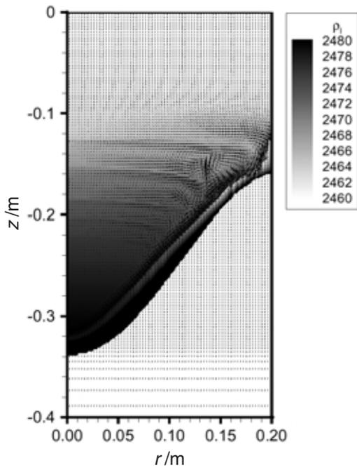
**Figure 2:** Liquid density ( $\rho_l$ ) and absolute velocity ( $v$ ) fields in the billet obtained in the full macrosegregation computation. The density field is shown only in the liquid and mushy zones ( $f_l > 0$ ).
