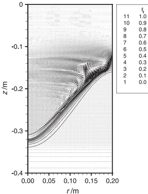
**Figure 3:** Relative velocity field ( $v-v_{cast}$ ) and liquid fraction isopleths in the billet obtained in the full macrosegregation computation
