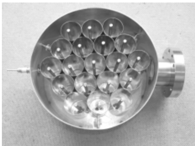
Slika 1: Fotografija nove magnetronske ionske črpalke Figure 1: Photograph of a new magnetron ion pump
