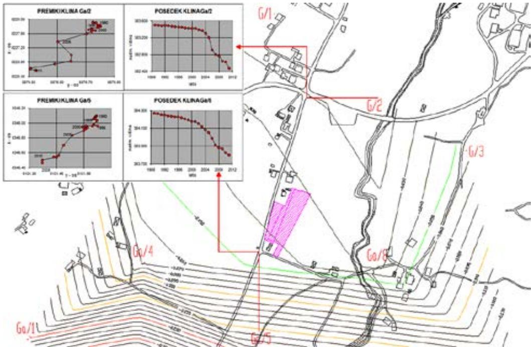
**Figure 7:** A map of the vertical movement isolines made based on the results of measurements in two periods of the observed points, and a graphical display of the individual points' movements.
