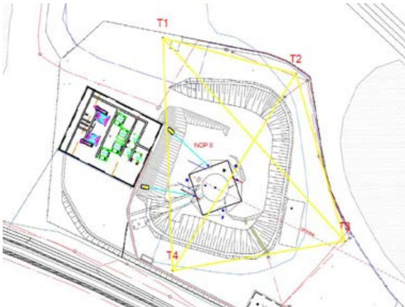
**Figure 5:** The situation in the area of the NOP II shaft with the observation pillars – points of the initial NOP II network.
