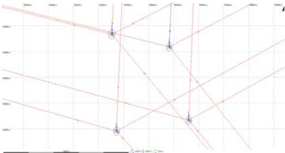
**Figure 11:** A graphical result of the GNSS processed points of the base observation network of the NOP II shaft.
