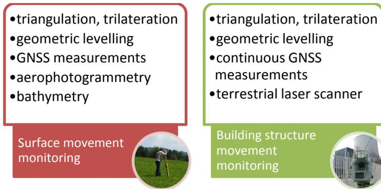
*Figure 2: The methods of monitoring movements and deformations on the area of The Velenje Coal Mine.*
