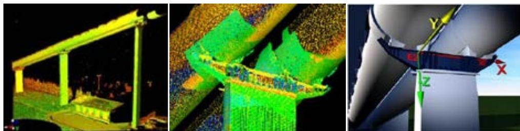
**Figure 12:** A scannogram of the observed building (left), a display of a certain detail (middle) and the final model of the building with the coordinate axes shown (right).
