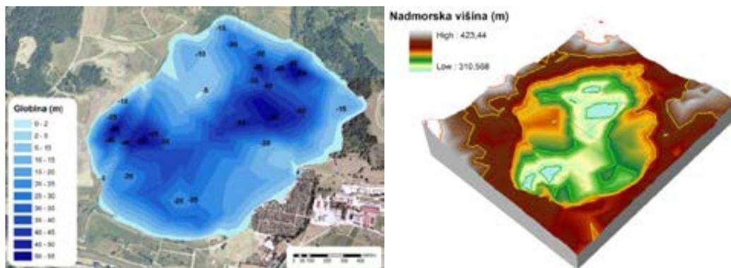
**Figure 9:** A bathymetric map (left) and a 3D model of the Velenje Lake lakebed (right).
