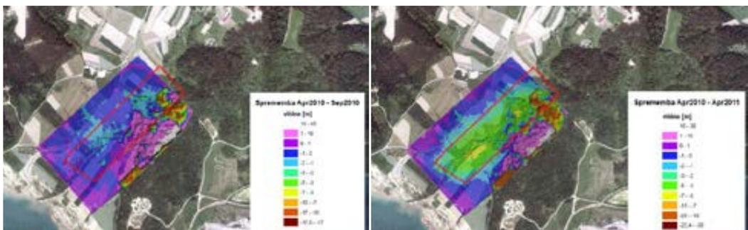
**Figure 8:** The results of changes in calculated terrain subsidence on the basis of aerophotogrammetry: April 2010–September 2010 (left) and April 2010–April 2011 (right).
