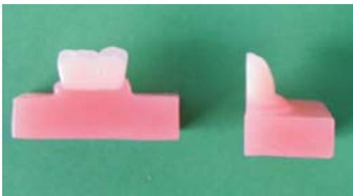
**Figure 1.** Acrylic model after its removal from the mould, prepared for microscoping
