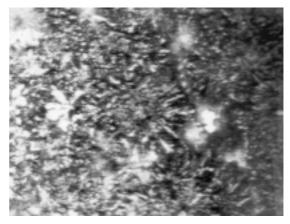
**Figure 7:** Microstructure of a white cast-iron sample, heat no. 4 with 8.72 wt. % vanadium, in as-cast condition, nital etched, 500× **Slika 7:** Mikrostruktura vzorca litine, talina 4 z 8,72 % vanadija, lito, jedkano z nitalom, 500-krat
