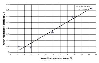
Figure 14: The effect of vanadium content in vanadium-alloyed, white cast-iron samples on the abrasion wear-resistance coefficient Slika 14: Vpliv vsebnosti vanadija na koeficient obrabne odpornosti litin
