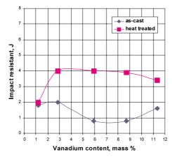
Figure 13: The effect of vanadium content on the impact resistance of as-cast and heat-treated white cast-iron samples, tested without notch Slika 13: Vpliv vsebnosti vanadija na žilavost litih in toplotno obdelanih litin; preizkušanci brez zareze
