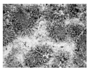
Figure 12: Microstructure of a white cast-iron sample, heat no. 5 with 11.32 wt. % vanadium, in heat-treated condition, nital etched,  $500 \times$  Slika 12: Mikrostruktura vzorca litine, talina 5 z 11,32 % vanadija, toplotno obdelano, jedkano z nitalom, 500-krat
