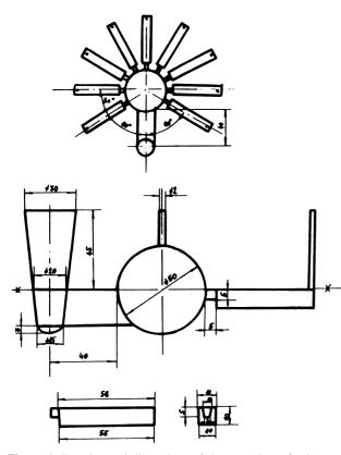
Figure 1: Drawing and dimensions of the cast pieces for impactresistance testing with the gating and risering systems
