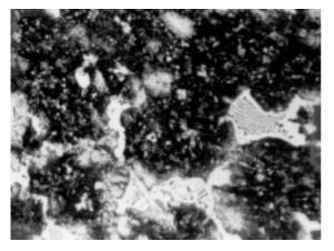
**Figure 6:** Microstructure of a white cast-iron sample, heat no. 3 with 5.94 wt. % vanadium, in as-cast condition, nital etched, 500× **Slika 6:** Mikrostruktura vzorca litine, talina 3 z 5,94 % % vanadija, lito, jedkano z nitalom, 500-krat
