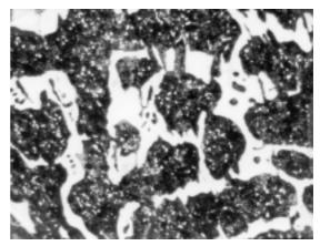
**Figure 9:** Microstructure of a white cast- iron sample, heat no. 1 with 1.2 wt. % vanadium, in heat-treated condition, nital etched, 500× **Slika 9:** Mikrostruktura vzorca litine, talina 1 z 1,2 % vanadija, toplotno obdelano, jedkano z nitalom, 500-krat
