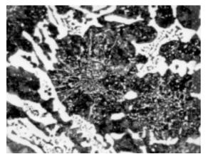
**Figure 10:** Microstructure of a white cast-iron sample, heat no. 2 with 2.86 wt. % vanadium, in heat-treated condition, nital etched, 500× **Slika 10:** Mikrostruktura vzorca litine, talina 2 z 2,86 % vanadija, toplotno obdelano, jedkano z nitalom, 500-krat
