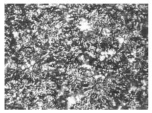
**Figure 8:** Microstructure of a white cast-iron sample, heat no. 5 with 11.32 wt. % vanadium, in as-cast condition, nital etched, 500× **Slika 8:** Mikrostruktura vzorca litine, talina 5 z 11,32 % vanadija, lito, jedkano z nitalom, 500-krat
