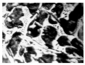
**Figure 5:** Microstructure of a white cast-iron sample, heat no. 1 with 1.2 wt. % vanadium, in as-cast condition, nital etched, 500× **Slika 5:** Mikrostruktura vzorca litine, talina 1 z 1,2 % vanadija, lito, jedkano z nitalom, 500-krat
