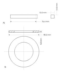
**Figure 2:** Drawing and dimensions of samples for testing of a) microstructure and hardness, and b) wear resistance **Slika 2:** Načrt in dimenzije vzorcev: a) za preiskavo mikrostrukture in
