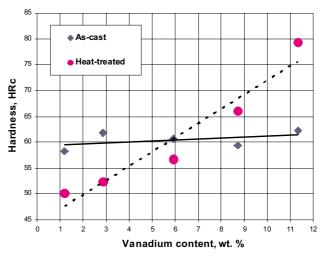
Figure 4: The effect of vanadium content on the hardness properties of white cast-iron samples in the as-cast and heat-treated conditions Slika 4: Vpliv vsebnosti vanadija na trdoto lite in toplotno obdelane bele litine
