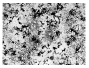
**Figure 11:** Microstructure of a white cast-iron sample, heat no. 4 with 8.72 wt. % vanadium, in heat-treated condition, nital etched, 500× **Slika 11:** Mikrostruktura vzorca litine, talina 4 z 8,72 % vanadija, toplotno obdelano, jedkano z nitalom, 500-krat
