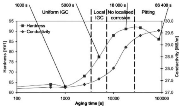
Figure 1: The dominant corrosion types in a material aged at 185 °C, according to<sup>5</sup>
