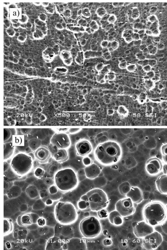
**Figure 3:** SEM micrographs of the surface of HC sample upon etching with NaOH: a) sample surface, b) transverse cut surface
